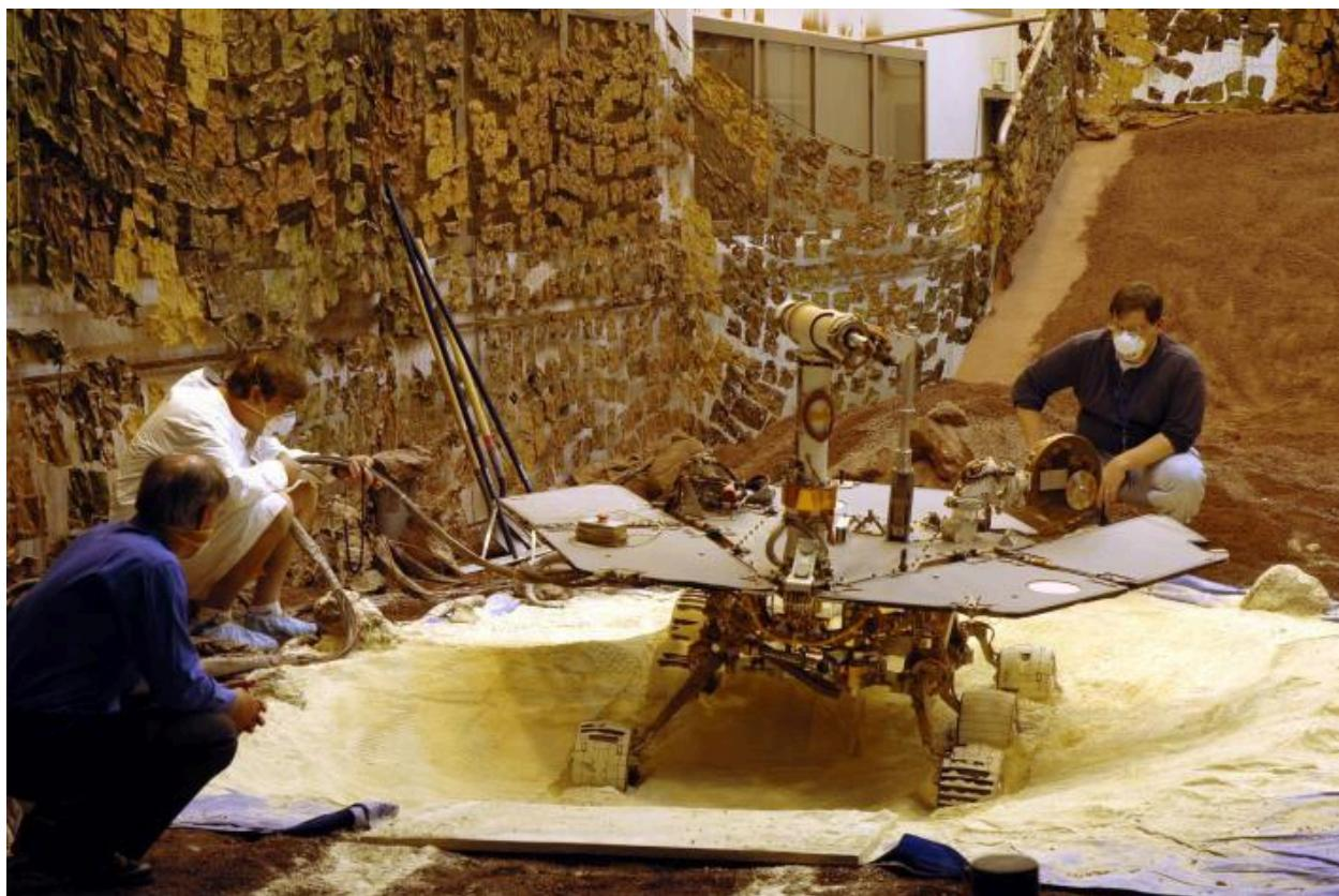
Rover engineers in JPL's In-Situ Instrument Lab check how a test rover moves in material chosen to simulate some difficult Mars driving conditions. Credits: NASA/JPL
